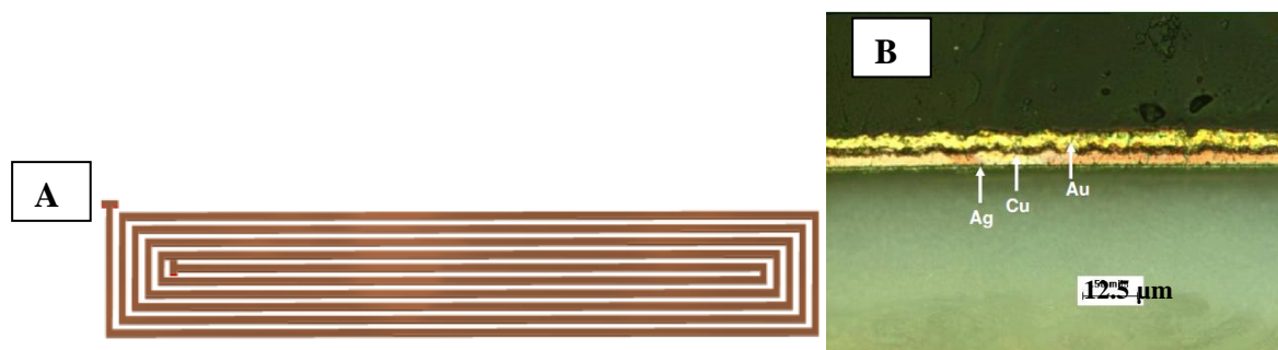
Figure 6 : (A) Spiral inductors, and (B) cross section of multilayered spiral inductors
