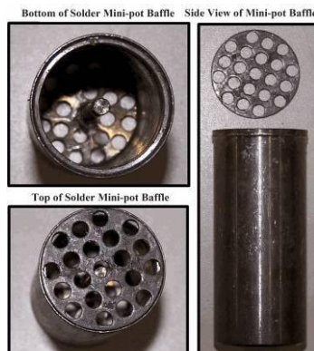
Figure 2 – Modified Solder Mini-pot Baffle
