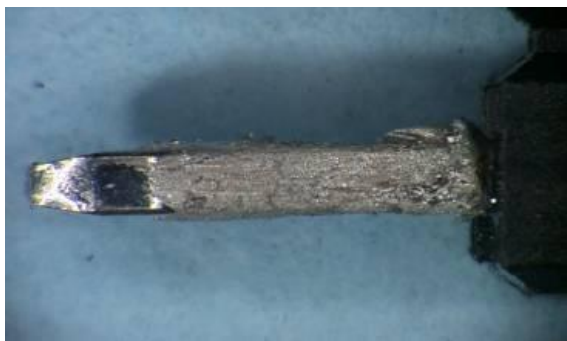
Figure 33. Typical appearance of fractured U-clip pins
