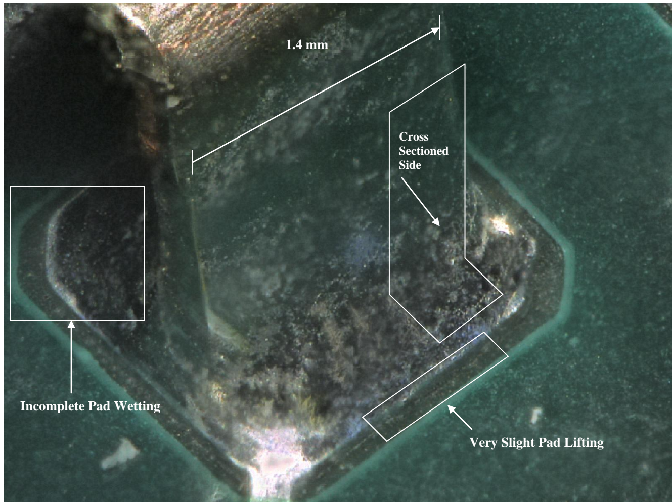
Figure 19 – PWB 50 - U59, Pin 3 (Au/Pd/Ni Finish)
