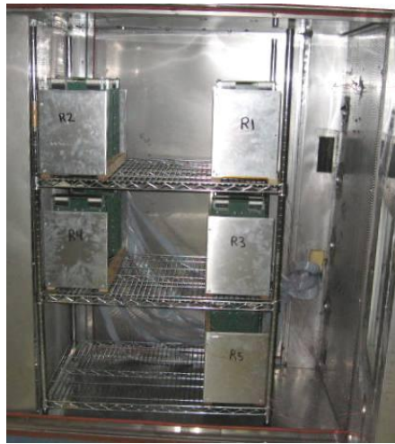
Figure 7 - ATC Chamber Showing Layout of Racks
