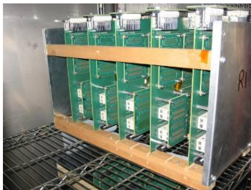
Figure 6 - "Metro2" Cards Mounted in a Rack for ATC Testing
