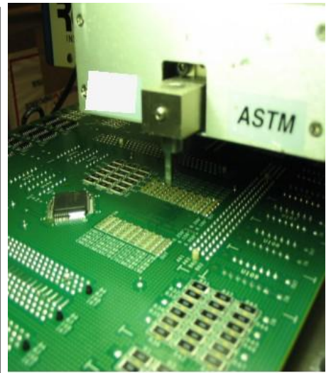
Figure 9: Shear force test set-up
