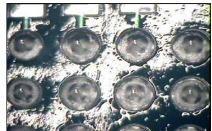
Figure 3: Rosin Wave Flux Residue
