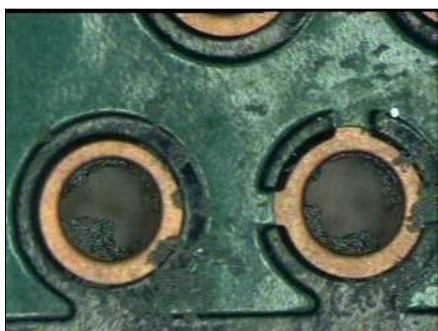
Figure 4: Smeared Solder Paste in Vias
