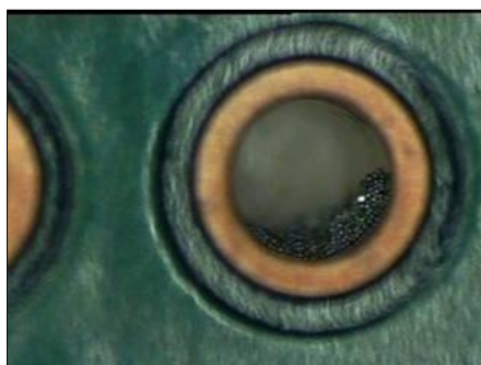
Figure 5: Solder trapped in PTH Via
