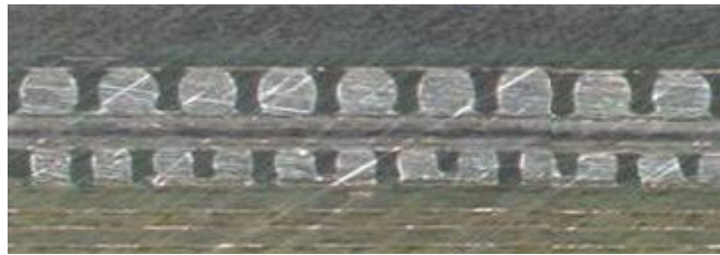
Figure 2b. Cross section image of an assembled PoP device (underfilled).
