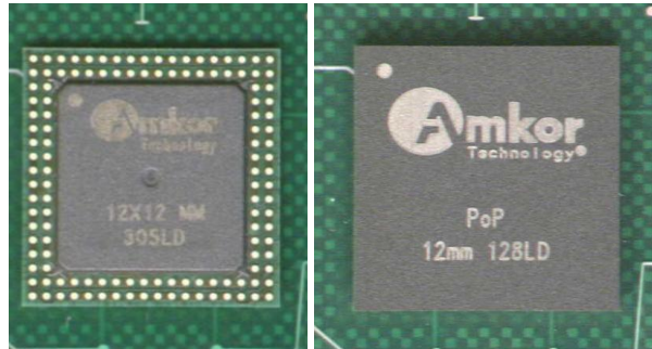
Figure 2a. Images of PoP packages, bottom package (left) and top package (right).
