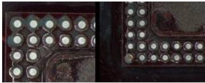
Figure 9. No cracks found on epoxy flux system.
