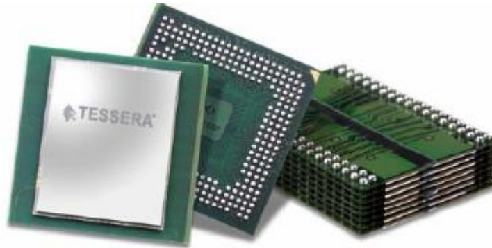
Figure 1. Vertically stacked \mu Z® FBGA for high-performance and higher density applications (Tessera).
