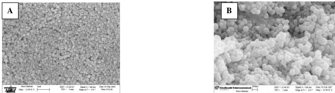
Figure 2: Larger area SEM image of composite specimens: (A) \text{BaTiO}_3 -epoxy (B) \text{BaTiO}_3 -fluoropolymer nanocomposites.
