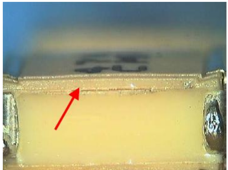
Figure 3. Cracks in the End of the Polyester Capacitor (After M. Wickham, et al. , 2003. [1]).
