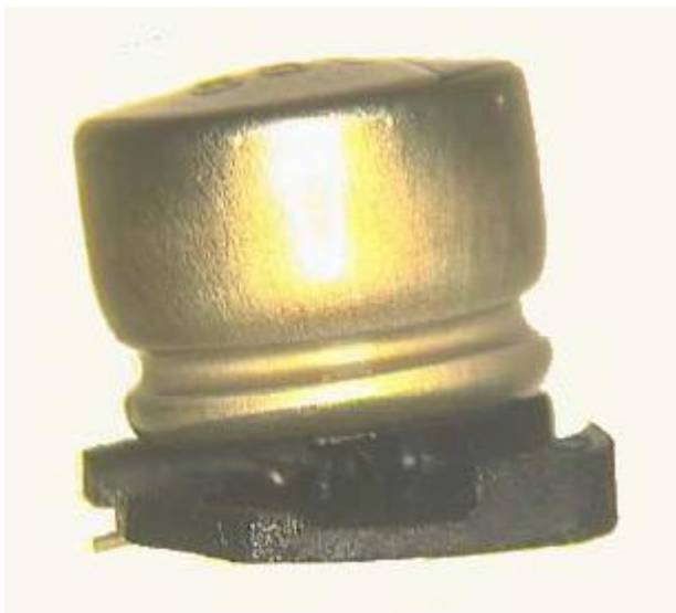
Figure 2. 100µF Electrolytic Capacitor after Pb-free reflow. Note temperature induced bulging of the can. (After M. Wickham, et al. , 2003. [1])
