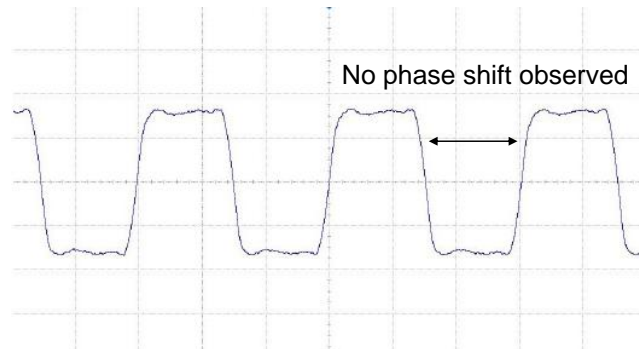
Figure 8. Suspect oscillator wave pattern shows no phase shifting.
