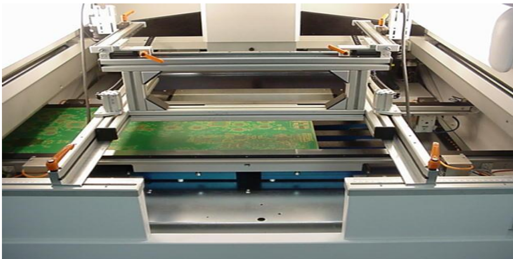
Figure 5. The experimental setup to determine stencil printing precision.
