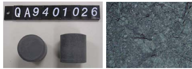
Figure 5 The homogeneous compliance of molding compound after grinding.
