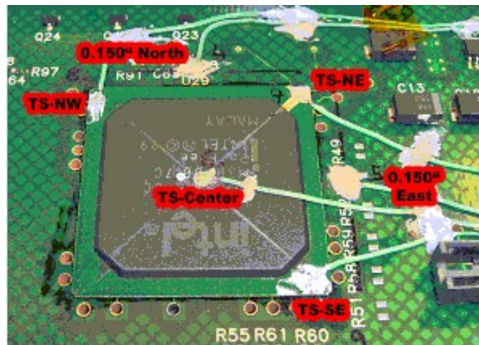
Figure 2: Topside thermocouple locations
