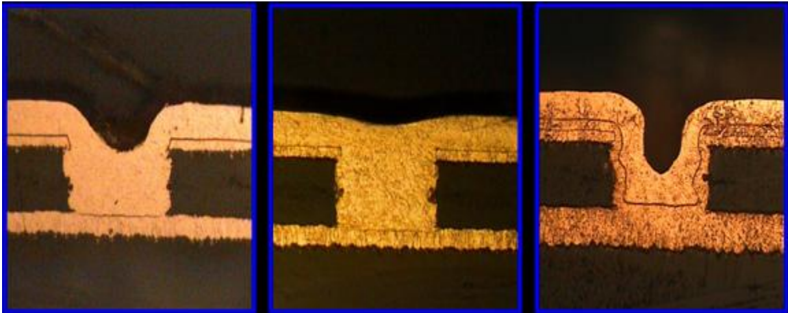
Figure 5 - Effect of Acid Copper Ratio (from left to right - ratios of 2, 1 and 0.5:1)
