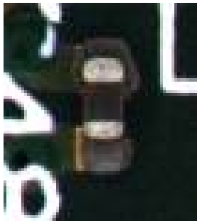
Figure 15: Defect image of one of the CC0402s.
