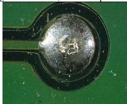
Figure 4 –No-clean, domed solder pad.
