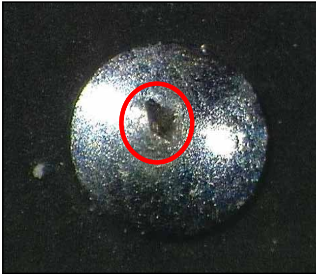
Witness mark of a 40 ° razor on a lead-free pasted solder “dome”, no-clean process
