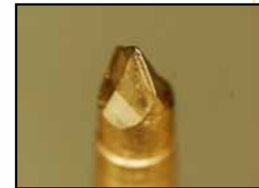
Same Probe after 67,900 cycles (flux has been cleaned)
