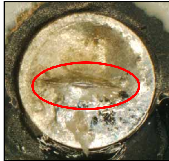
Witness mark of a 150° razor sharp tip on lead-free pasted test pad, no-clean process
