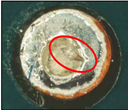
Witness mark of a 90 ° razor on a lead- free pasted via, no- clean process.
