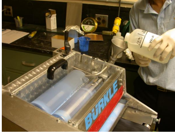
Figure 1 Clean Up of Waterbased Photoresist with Soap and Water
