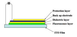
Fig. 2 Basic construction of the printed EL
