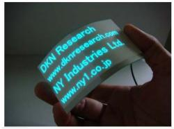
Fig. 6 Example of the flexible EL maid by all screen-printing process
