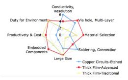
Fig. 1 Comparison of the circuit manufacturing processes
