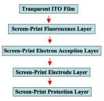
Fig. 5 Basic process of the printed EL
