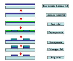
Fig. 4 Basic patterning process of the copper foil circuits
