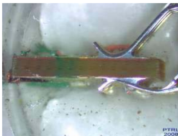
Figure 9 No copper plane beneath colder pads
