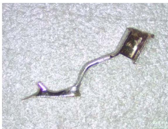
Figure 7 Typical pin with copper pad attached
