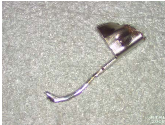
Figure 8 Typical pin with a solder-lead interface failure
