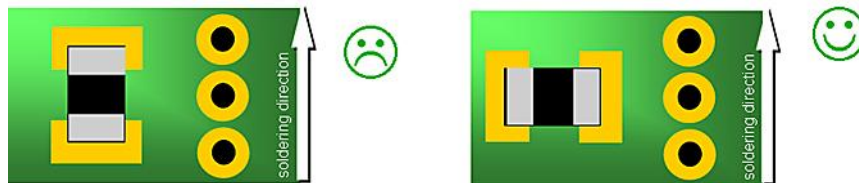
Figure 6 – Alignment of neighbouring SMD components
