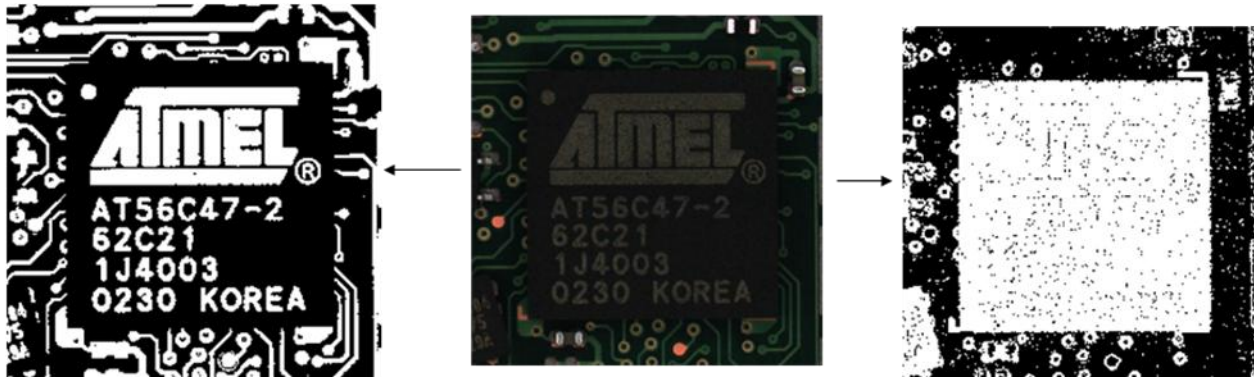
Figure 4 – Example of how a system with a single camera and one lighting mode can use color to separate a parts from its background. The middle image shows a dark black BGA on a primarily dark green background. The left image shows the results of a standard image contrast enhancement technique, which results in an undesirable highlighting of the text on the part and traces and vias on the board rather than the part boundaries. The results from a more sophisticated image analysis algorithm, generated from Landrex Optima™ 7200 series and shown on the right, can delineate the part neatly from the background. The main point is that more sophisticated algorithms are required for a single color camera system with fixed lighting.
