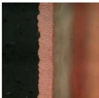
Figure 7 - Cross section of 0.2mm Through Hole in 1.6 mm Panel Plated at 1.0 ASD
