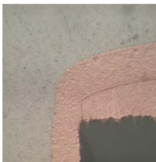
Figure 9 – Hi Throw DC Process, Plating at 1.0 ASD; Cross Section of 0.5 mm through hole after 6x Solder Shock
