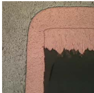
Figure 12 – HT Process, Plating at 35°C, 2.0 ASD; Cross Section of 0.5 mm through hole after 6x Solder Shock
