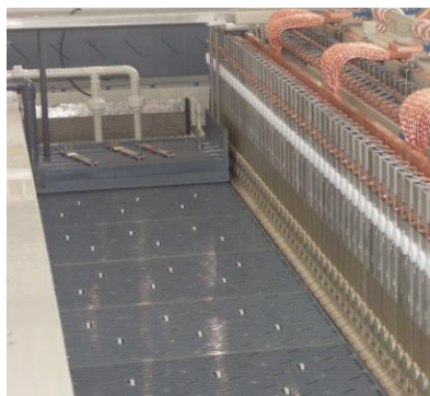
Figure 5 – Open View of Horizontal Conveyerised Copper Plating Module
