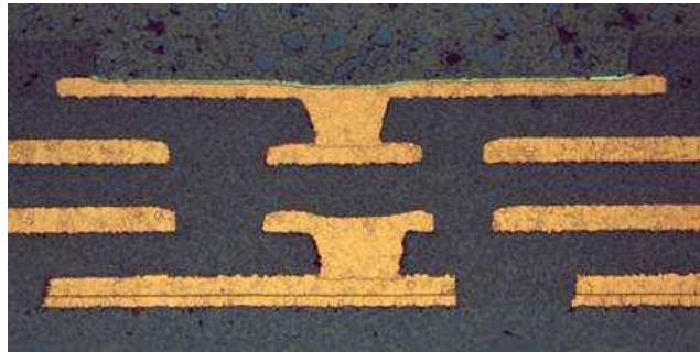
Figure 2 – IC Substrate with Copper Filled Build-Up Layers.
