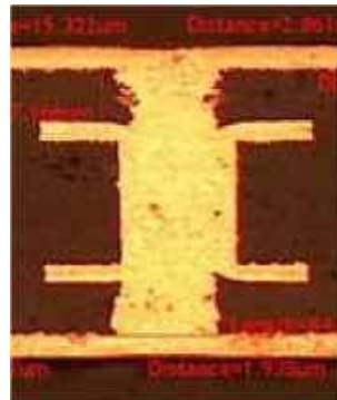
Figure 11 - Core filled with electrolytic copper followed by filled BMV with minimum surface plated copper.
