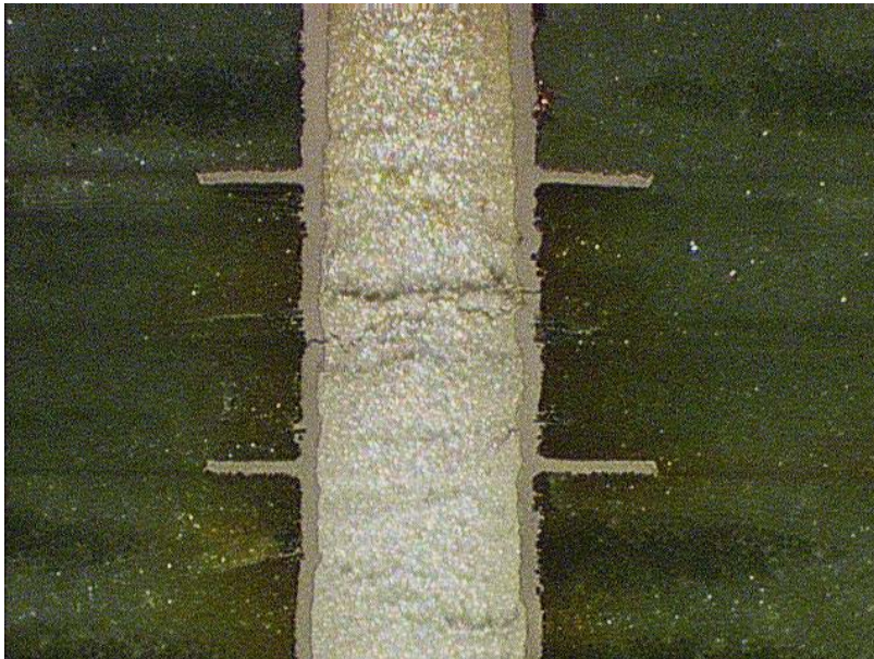
Figure 7: Micro section of via with failure in region where non-functional pads have been retained.
