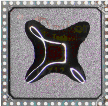
Dispense X-Pattern on Mold Cap of bottom package
