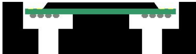
Figure 6. Cross section of pallet pocket design with PSvFBGA in place.
