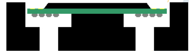
Sectioned view of pocket with pedestal and relief at solder balls
