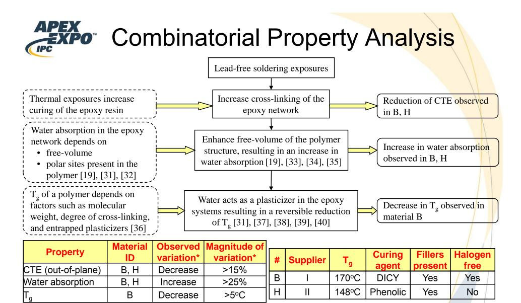
• Variation refers to the difference of measurement results between control and 6X reflowed samples
