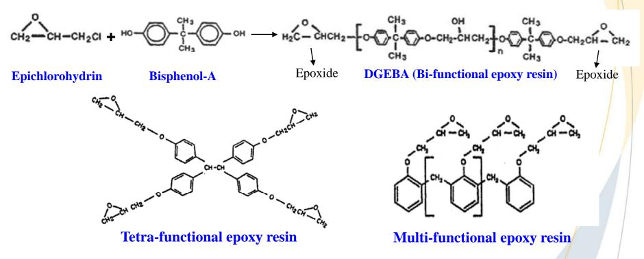
The epoxy groups react in subsequent resin polymerization and result in curing of the resin system
