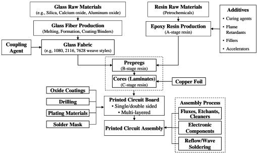
Figure 1: FR-4 printed circuit assembly fabrication
