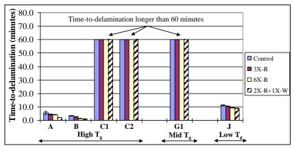
Figure 6: Effect of lead-free soldering exposures on T-260
