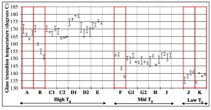
Figure 3: Effect of lead-free soldering exposures on T<sub>g</sub> of the laminates
