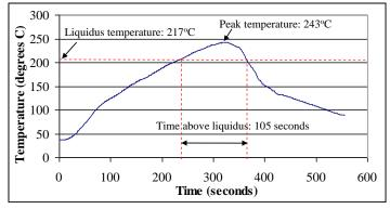
Figure 2: Lead-free reflow profile used for the exposures
