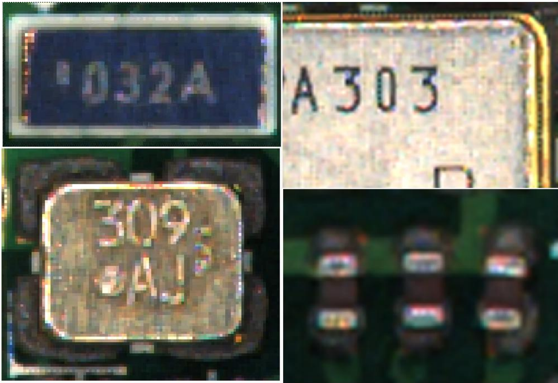
Figure 17- Examples of color artifacts on real parts on PCB boards. These images were created with one of the most sophisticated color recovery algorithms. This demonstrates that color artifacts cannot be avoided and, therefore, must be accounted for in the inspection system's subsequent image processing.
