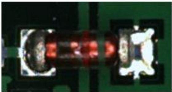
Figure 1: This is a picture of MELF diode on a reflowed board. The color bands indicate its value. Color processing is important in this example to know if the correct part has been placed. (Note that this part has a tombstone defect which caused a solder defect on the right side)
