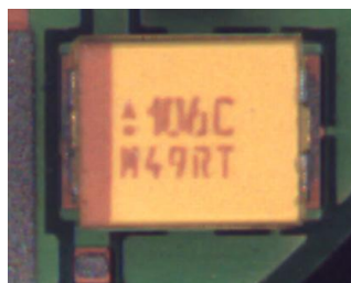
Figure 11- Example of good color discrimination for a yellow tantalum capacitor with a red orientation mark.
