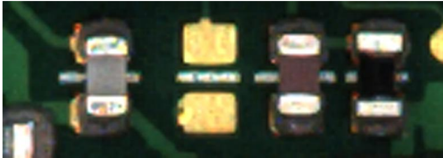
Figure 12: Example of good color discrimination between the end caps, paste and pads.
