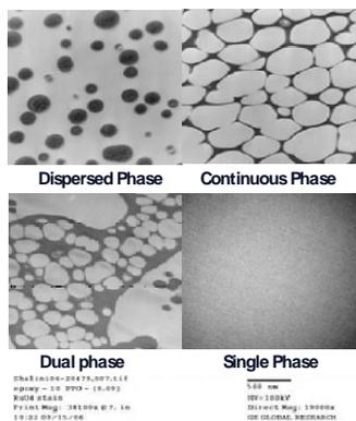
Figure 2. Microstructure of various PPE/Epoxy resins
