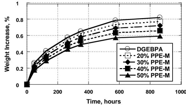
Figure 8. Effect of PPE-M on water uptake of DGEBA
