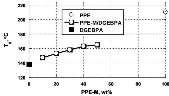
Figure 4. Effect of PPE-M on  $T_g$  of DGEBA
