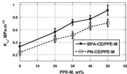
Figure 14. Effect of PE-M on Fracture Toughness of BPA-CE and PN-CE
