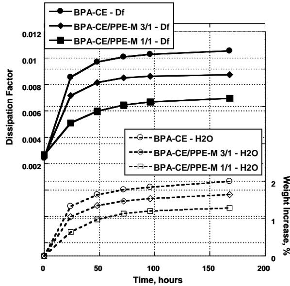
Figure 17. Effect of Moisture Absorption on Loss Tangent of BPA-CE
