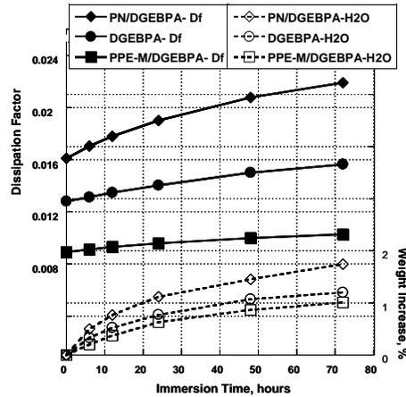
Figure 12. Effect of Moisture Absorption on Loss Tangent
