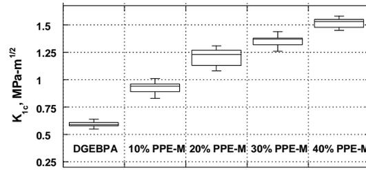
Figure 7. Effect of PPE-M on Fracture Toughness of DGEBA
