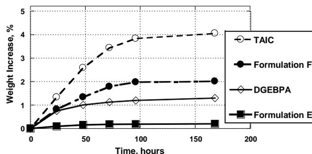
Figure 19. Moisture Uptake in TAIC and TBS/DVB Castings
