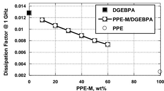
Figure 6. Effect of PPE-M on the Loss Tangent of DGEBA
