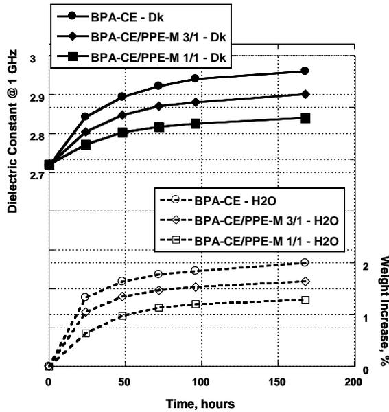
Figure 16. Effect of Moisture Absorption on Dielectric Constant of BPA-CE
