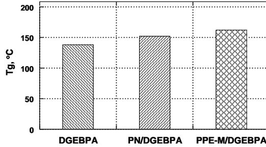
Figure 9. Effect of PN and PPE-M on Glass Transition Temperature
