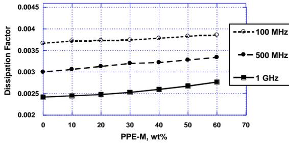
Figure 16. Loss Tangent versus PPE-M Levels in BPA-CE
