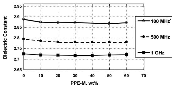
Figure 15. Dielectric Constants versus PPE-M Levels in BPA-CE
