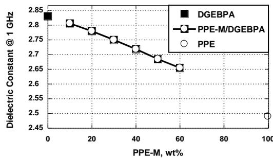
Figure 5. Effect of PPE-M on the Dielectric Constant of DGEBA
