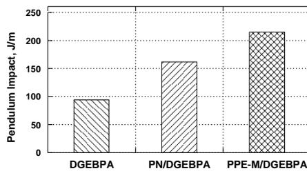
Figure 10. Effect of PN and PPE-M on Pendulum Impact
