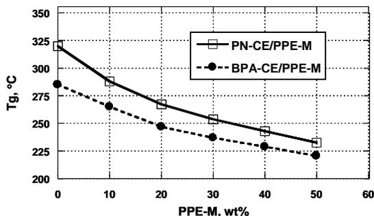
Figure 13. Effect of PE-M on Tg of BPA-CE and PN-CE Castings
