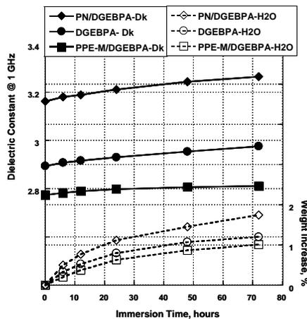
Figure 11. Effect of Moisture Absorption on Dielectric Constant
