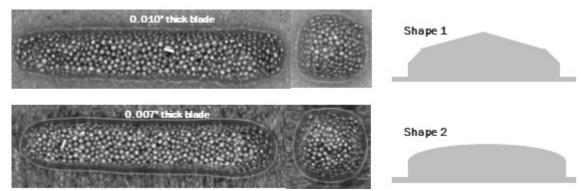
Figure 15. Optical image of rectangular and circular shape aperture showing the paste deposit shape.
