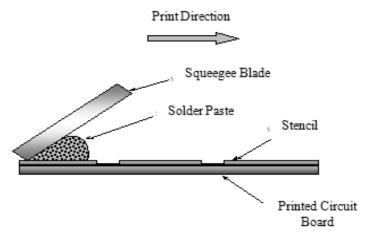
Figure 2. Typical printing process
