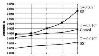
Figure 8. Deflection of base for different thickness active and static state
