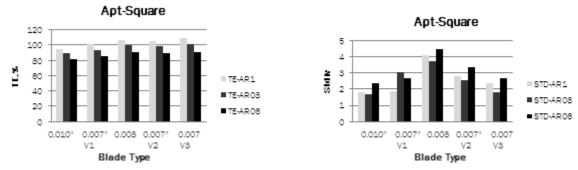
Figure 16. Effect of blade thickness on TE and Standard Deviation for square aperture
