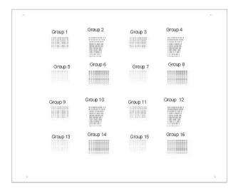
Table 2. Aperture layout Aperture shape Aperture Group # orientation No effect 1,3,9,11 Square Circular No effect 5,7,13,15 Rectangular Vertical 2,4,10,12 Rectangular Horizontal 6,8,14,16
