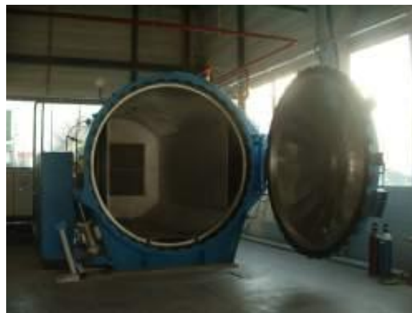
Autoclave used for PVB processes
