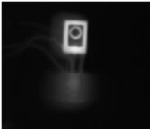
Figure 2. Through-hole transistor in TO-32 case with maximum case temperatures of 163°C.
