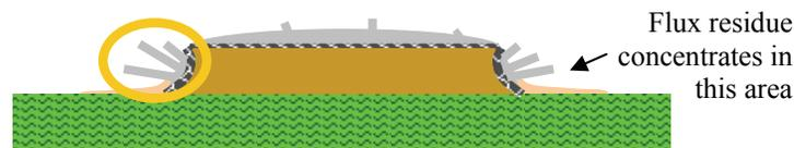
Figure 5. Schematic indication of pattern of whisker growth.
