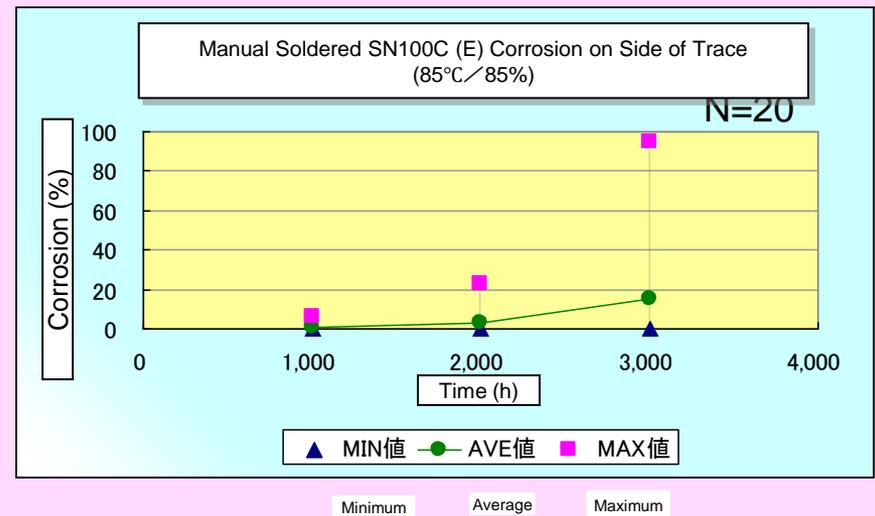
Corrosion with Halogen-Free SN100C (E) is
