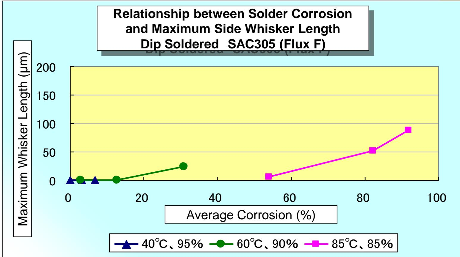
Maximum whisker length is proportional to the extent of solder corrosion
