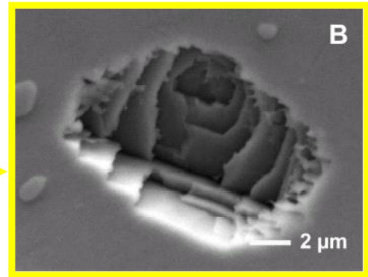
**CRYSTALLOGRAPHICALLY-FACETTED VOID FORMATION IN THE MATRIX OF LEAD-FREE SOLDER JOINTS** S. Belyakov, H V Atkinson and S P A Gill, Department of Engineering, University of Leicester. JEMS-1777
