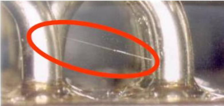
Risk of current leakage and shorting due to bridging of adjacent conductors
