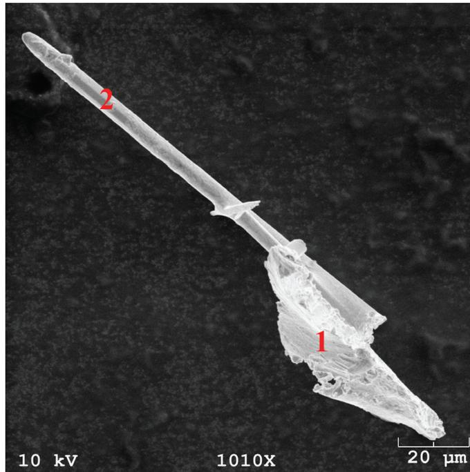
**Figure 6:** Scanning electron micrograph of the microbridge fragment retrieved from the short circuit site shown in Figure 2. Note that the portion of the fragment labeled with the “2” has a distinct needle like shape. The irregular mass of material marked by the “1” at the lower right was part of the conical base that joined the needle like segment to one of the two solder joints. EDS spectra obtained from the two labeled locations are shown in Figures 7 & 8.
