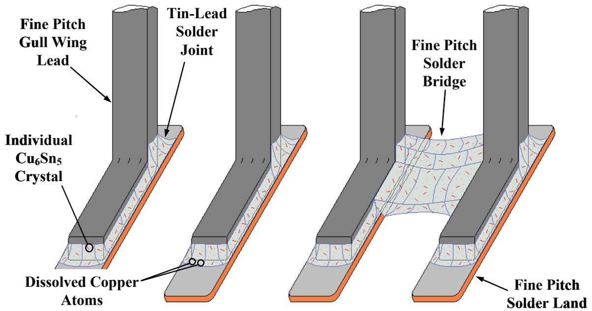
**Figure 14A:** The reflowed condition of a solder paste bridge between fine pitch gull wing leads. The solder in the joints and the bridge is already saturated with copper and some  $\text{Cu}_6\text{Sn}_5$  crystals.
