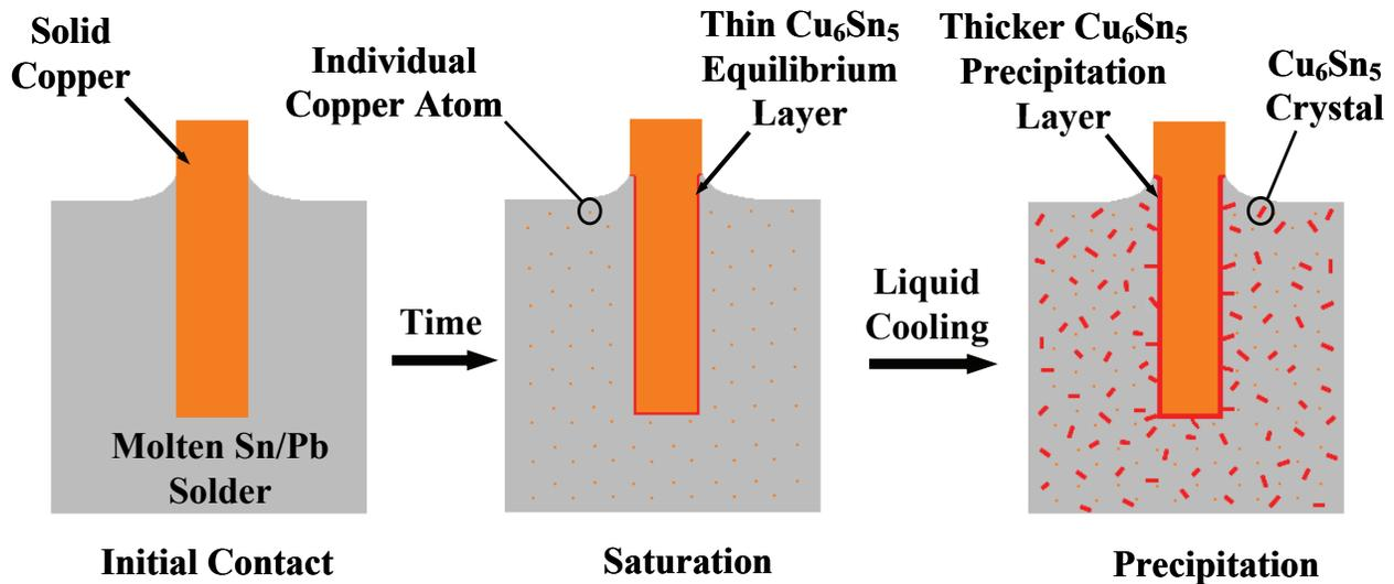
**Figure 9:** Illustration of the mechanism by which  $\text{Cu}_6\text{Sn}_5$  crystals form within a volume of molten solder. Given enough contact time, copper atoms from an immersed copper structure will dissolve into the molten solder and saturate it.  $\text{Cu}_6\text{Sn}_5$  crystals will then precipitate out at the copper interface, and within the solder itself, as the saturated solder cools.
