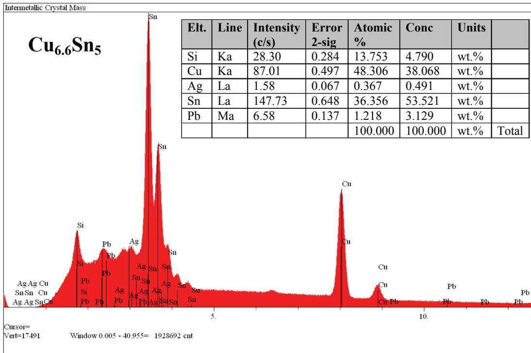
**Figure 25:** EDS spectrum obtained from the site outlined by the yellow box on the cluster of intermetallic crystals shown in Figure 23. The metallic crystal that generated this spectrum was composed primarily of copper and tin, and relatively little silver (Ag) or lead (Pb). The copper/tin stoichiometric ratio at this location was 6.6 to 5 respectively, again a close match for Cu<sub>6</sub>Sn<sub>5</sub>. The silicon peak was attributed to the PWB surface in the background.
