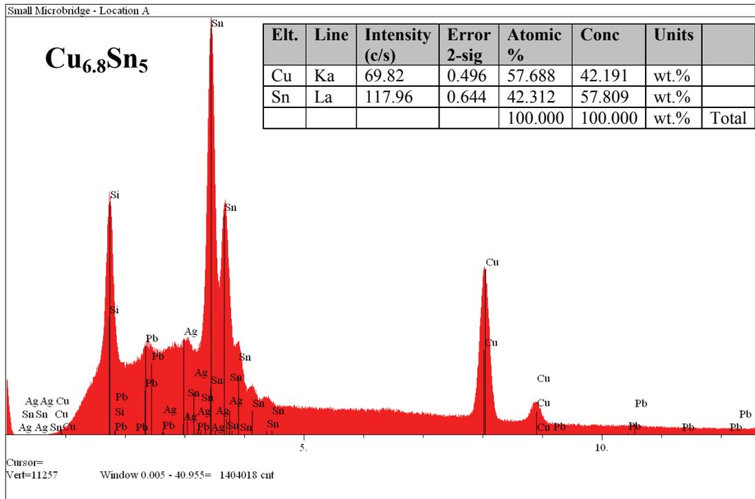
**Figure 24:** EDS spectrum obtained from Location A in Figure 23. This single crystal surface exhibited virtually no silver (Ag) or lead (Pb). The copper/tin stoichiometric ratio at this location was 6.8 to 5 respectively, again a close match for  $\text{Cu}_6\text{Sn}_5$ . The silicon peak was attributed to the PWB surface in the background.
