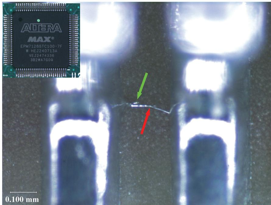
**Figure 2:** This microbridge (red arrow) was found on an assembly that had not yet been conformal coated. It consisted of two needle like segments that met at a slight angle near the middle of the 0.2 mm gap between 0.5 mm pitch gull wing leads (actual QFP device at upper left). A green arrow highlights a smaller needle like protrusion that extended out of the cone shaped base on the left end of the microbridge.
