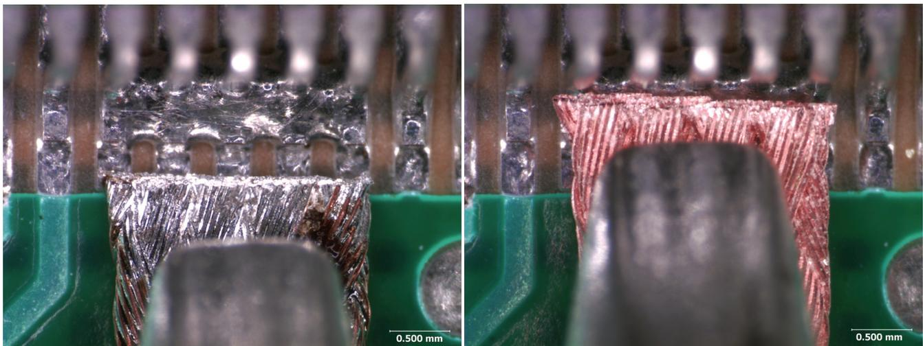
**Figure 29:** Lab experimentation indicated that microbridges were more likely to form when the desoldering braid was applied along the extreme outside edge of the printed wiring board lands, and when the desoldering braid was already partially soaked with solder (left). No microbridges formed when fresh desoldering braid was applied directly to the bridge site, in conjunction with the rework method outlined in Figure 28.
