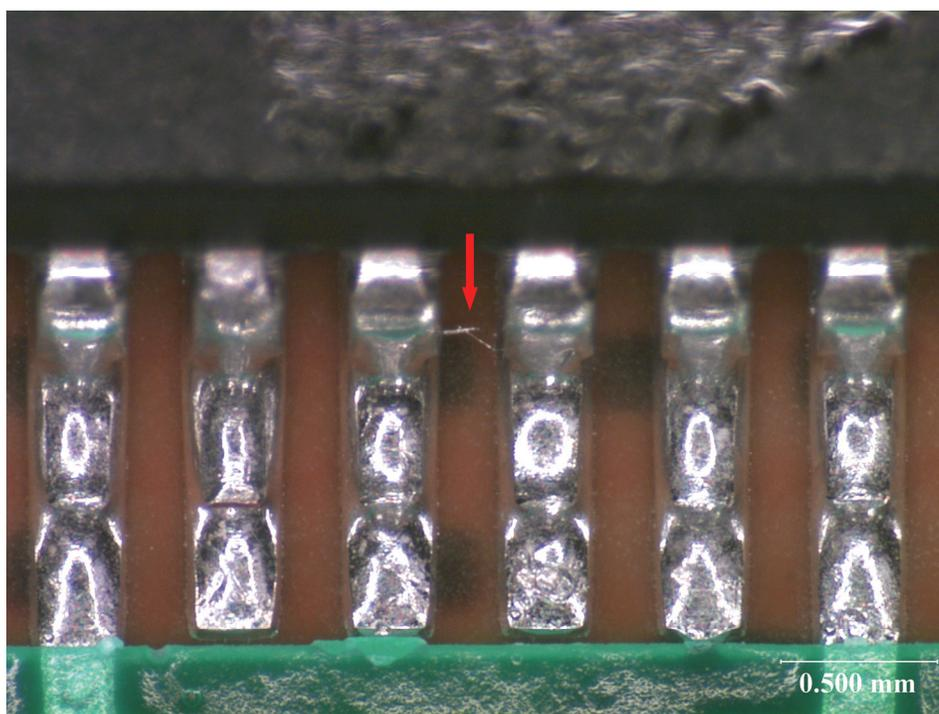
**Figure 11:** Production microbridge (red arrow) consisting of multiple needle like segments found in the 0.15 mm gap between 0.5 mm pitch gull wing leads on an Sn62/Pb36/Ag2 paste assembly. The above solder joints were hand reworked.
