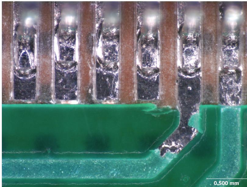
**Figure 28:** The reworked fine pitch solder bridge site from Figure 27. No microbridges formed during the rework process.
