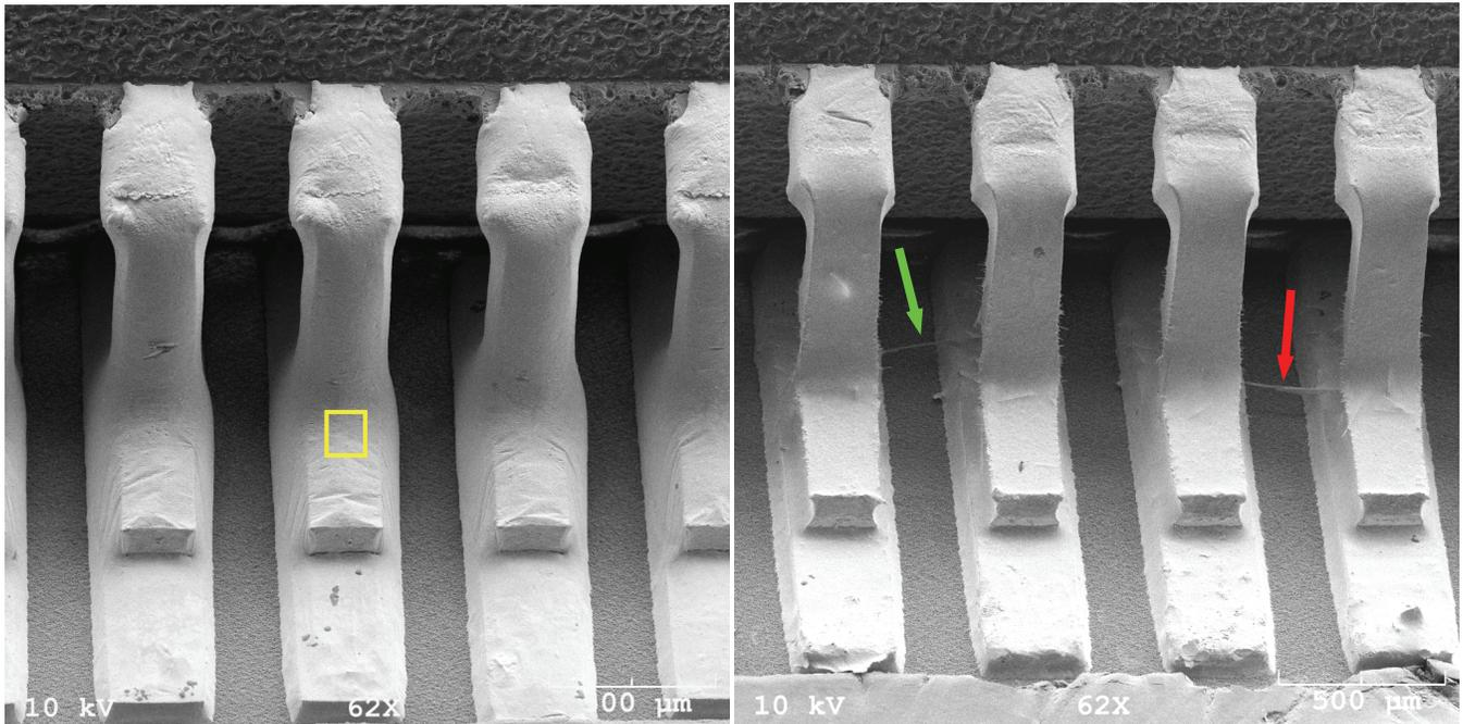
**Figure 18:** Scanning electron micrographs of as reflowed solder joints (left) and reworked solder joints (right) from the row of solder joints shown in Figure 16. The red and green arrows highlight the same two microbridges first shown in Figure 17. The yellow box on the left shows the location from which the EDS spectrum in Figure 19 was obtained.
