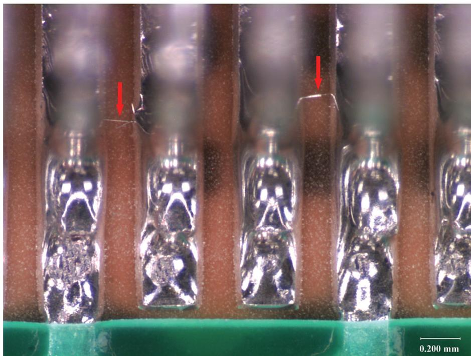
**Figure 10:** Production microbridges (red arrows) consisting of single needle like segments found in the 0.15 mm gaps between 0.5 mm pitch gull wing leads on an Sn62/Pb36/Ag2 paste assembly. The above solder joints were hand reworked.
