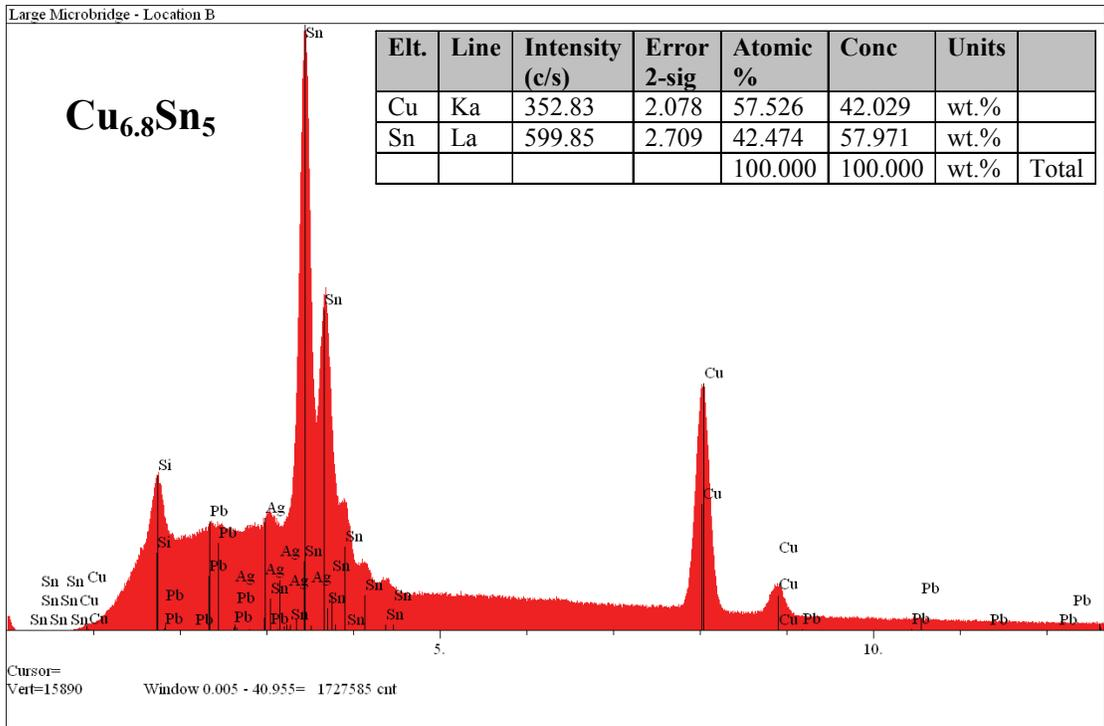
**Figure 22:** EDS spectrum obtained from Location B in Figure 20. This single crystal surface exhibited virtually no silver (Ag) or lead (Pb). The copper/tin stoichiometric ratio at this location was 6.8 to 5 respectively, a close match for  $\text{Cu}_6\text{Sn}_5$ . The silicon peak was attributed to the PWB surface (i.e. glass fibers) in the background.
