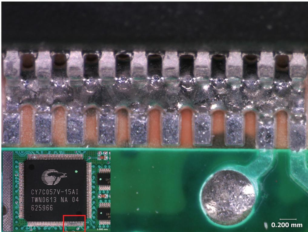
**Figure 15:** Solder bridges made by applying excess Sn62/Pb36/Ag2 solder paste to the 0.2mm gaps between the 0.5 mm pitch gull wing leads of the inset component. The paste was subjected to a normal reflow profile in a hot air belt oven. The bridges were located in the area outlined in red.
