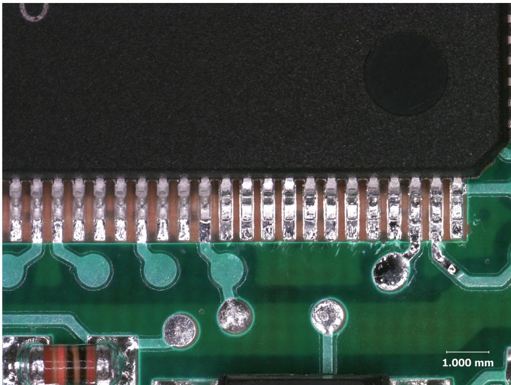
**Figure 16:** This overall view of the bridge site shown in Figure 15 was taken after the bridged joints had been reworked with desoldering braid and a soldering iron. Note that the reworked solder joints on the right are bright and shiny, while the as reflowed joints on the left are somewhat duller.
