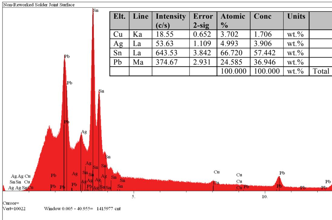
**Figure 19:** EDS spectrum obtained from the as reflowed solder joint surface outlined by the yellow box in Figure 18. The Sn62/Pb36/Ag2 solder paste that formed this joint absorbed approximately 1.7% copper (Cu) by weight.
