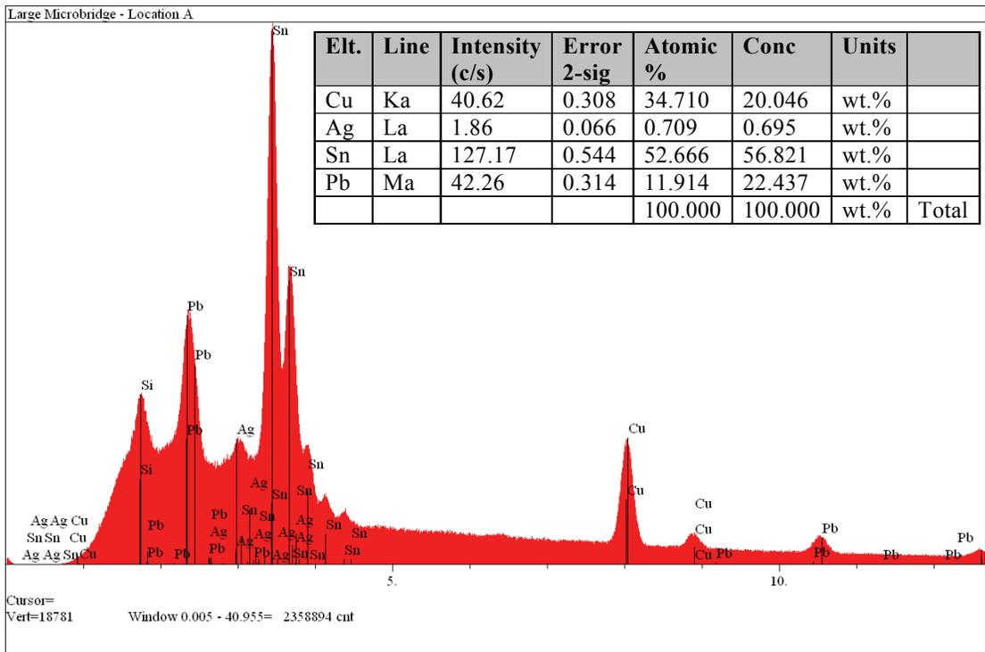
**Figure 21:** EDS spectrum obtained from Location A in Figure 20. The combination of elements present at this location confirmed the initial visual assessment that this site consisted of a subsurface bundle of  $\text{Cu}_6\text{Sn}_5$  crystals covered by a thin film of Sn62/Pb36/Ag2 solder.
