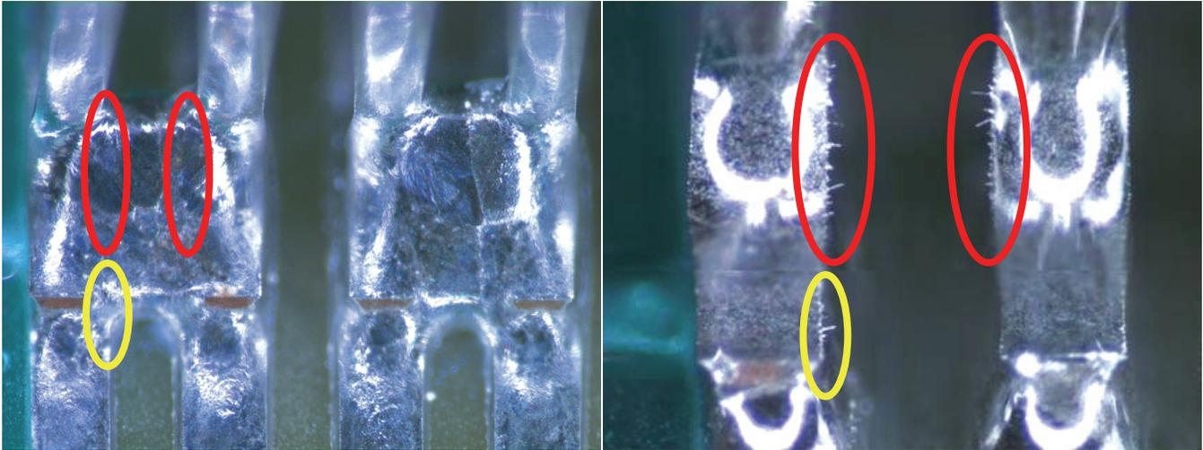
**Figure 26:** Actual production Sn63/Pb37 solder paste bridges located in the 0.2 mm gap between adjacent 0.5 mm pitch gull wing leads (left). The same locations outlined on the left are shown again on the right after being hand reworked by a production operator with a soldering iron and desoldering braid. Clusters of  $\text{Cu}_6\text{Sn}_5$  crystals can be seen along the edges of both component leads.
