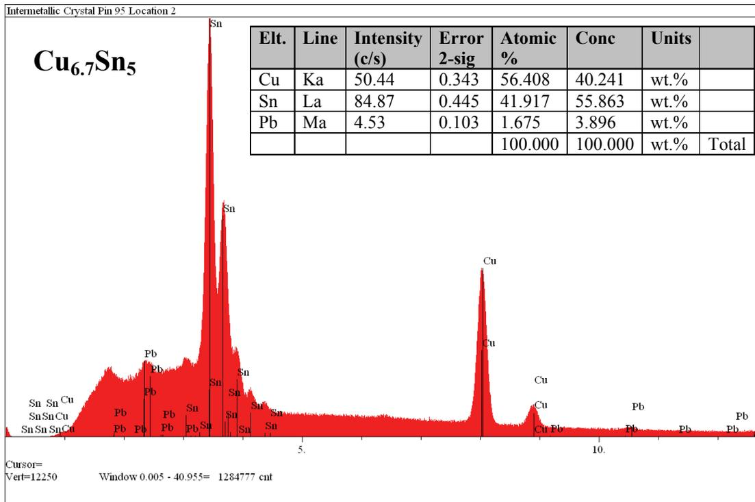
**Figure 8:** EDS spectrum obtained from Location 2 in Figure 6. This material from one of the needle like segments of the microbridge was composed primarily of copper (Cu) and tin (Sn), with only a trace of lead (Pb). The stoichiometric ratios of the copper and tin, which are shown at the upper left, closely approximated the atomic formula for Cu<sub>6.7</sub>Sn<sub>5</sub>, a known copper/tin intermetallic compound with an orthorhombic (i.e. needle like) structure.
