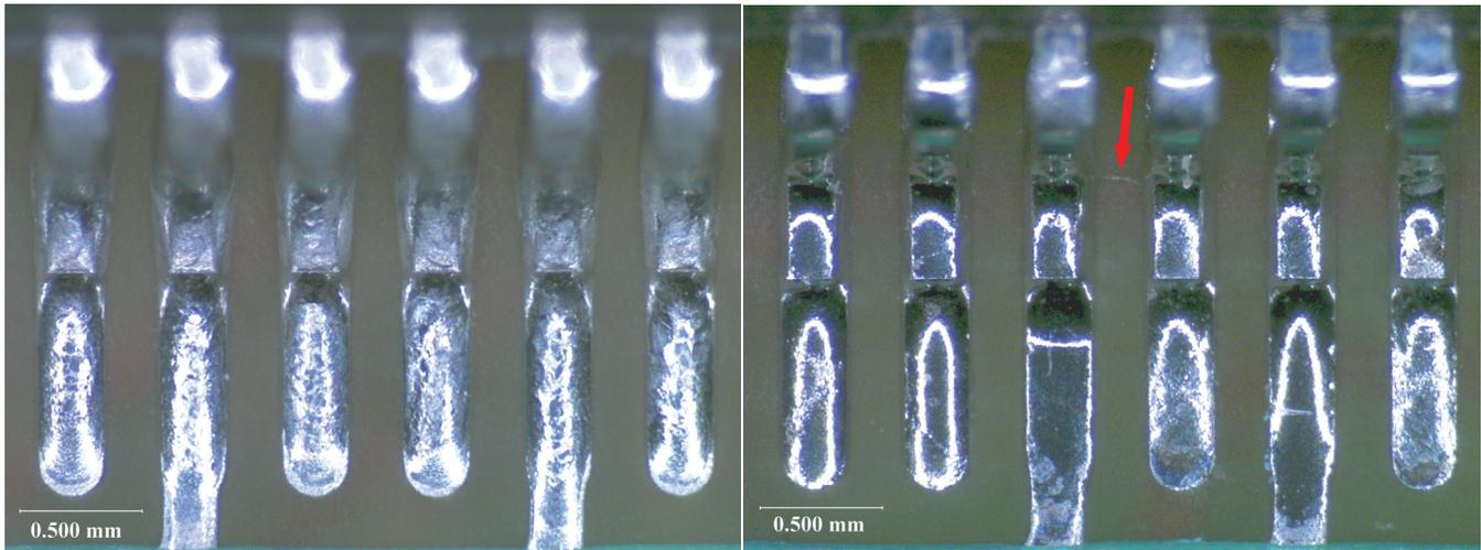
**Figure 4:** Hot air reflowed QFP solder joints (left), and hand reworked QFP solder joints (right). The red arrow highlights the microbridge shown in Figure 2. The solder joints from the paste reflow process were slightly duller, and had a crusty patina. The hand reworked solder joints were uniformly smooth, bright, and shiny.
