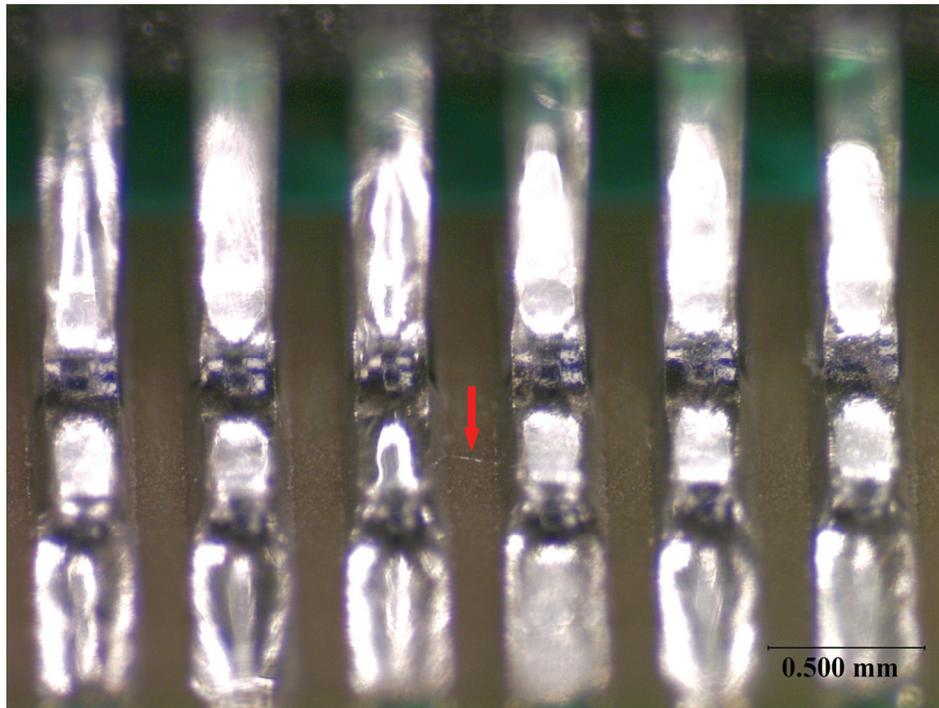
**Figure 12:** Production microbridge (red arrow) consisting of a single needle like segment found in the 0.15 mm gap between 0.5 mm pitch gull wing leads on an Sn63/Pb37 paste assembly. The above solder joints were hand reworked.
