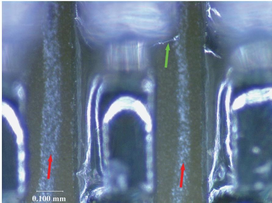
**Figure 3:** Two red arrows highlight probe scratch marks in the printed wiring board surface in the 0.2 mm gaps between 0.5 mm pitch QFP gull wing leads. These scratch marks were found on the same component, and just a few solder joints away from, the microbridge shown in Figure 2. The green arrow highlights the remnant of a microbridge broken by the probe tip.
