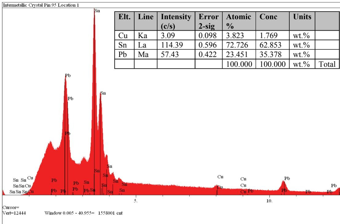
**Figure 7:** EDS spectrum obtained from Location 1 in Figure 6. This material from the conical base of the microbridge was composed mainly of tin (Sn) and lead (Pb). The weight percents of these two elements approximated the values expected for the Sn63/Pb37 solder that had been used on the assembly. The remainder of this material, nearly 1.8% by weight, was copper (Cu).
