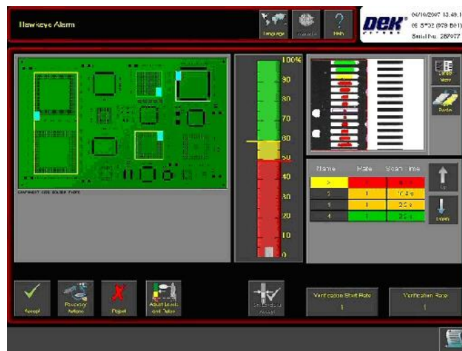
Figure 1 – Post-print inspection with built-in analysis and Good-board/Bad-board signaling.
