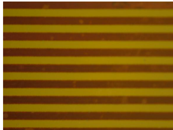
Figure 4b: Fail – Flux residue detected at 40X
