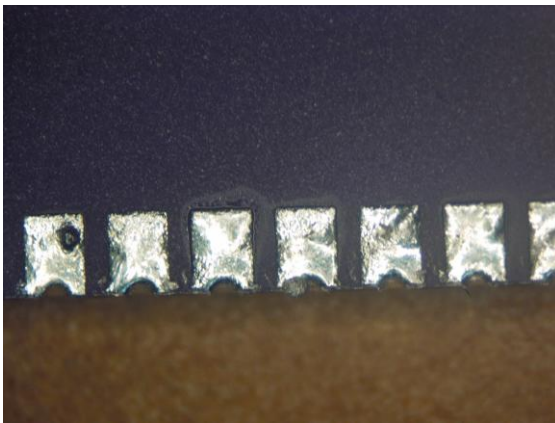
Figure 4a: Fail - Flux residue detected at 40X
