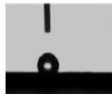
Fluorocarbon coating Contact angle : 95^\circ
