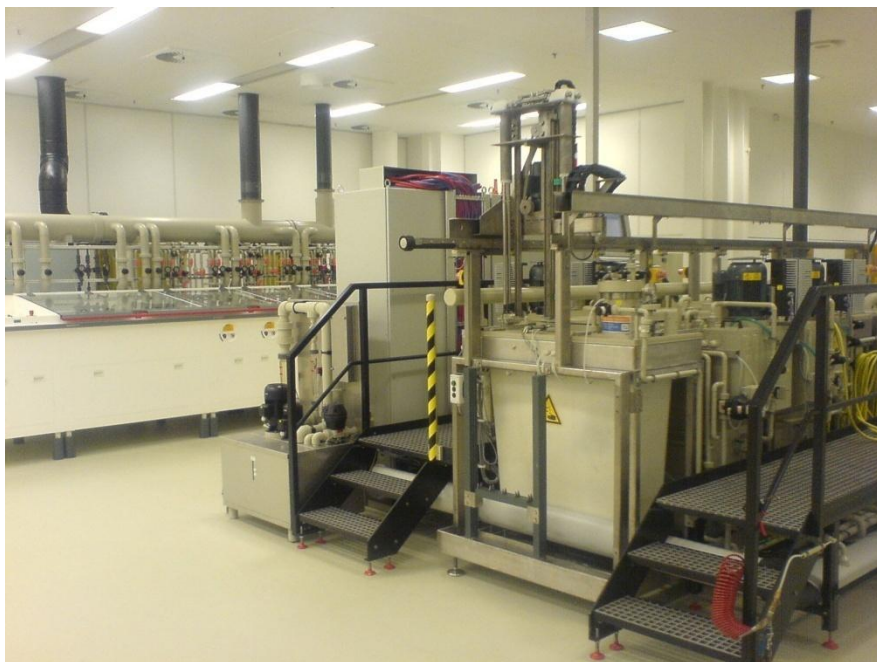
Single Board Plating Line : High uniformity across the panel
