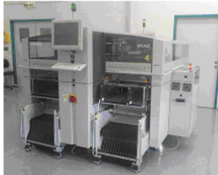
Figure 6 – SEAS SIPLACE X2 high-speed assembly machine
