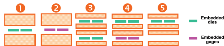
Figure 16 – Overview of the 5 types of embedded structures.
