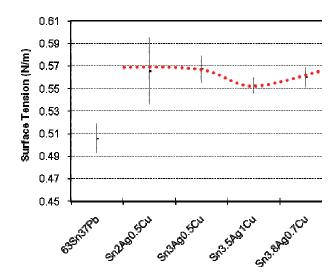
Fig. 2 Surface tension of Sn63Pb37 and SnAgCu alloys determined at 245°C and 260°C, respectively [2].
