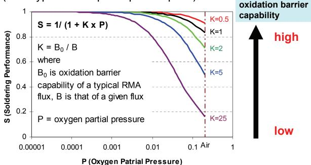
P. Jaeger and N.-C. Lee, "A Model Study of Low Residue No-Clean Solder Paste", in Proceeding of Nepcon West, Anaheim, CA, 1992. Fig. 9 Soldering performance versus oxidation barrier capability versus oxygen partial pressure [6].
