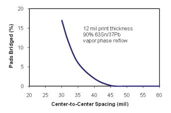
Fig. 8 Effect of center-to-center spacing on bridging [5].
