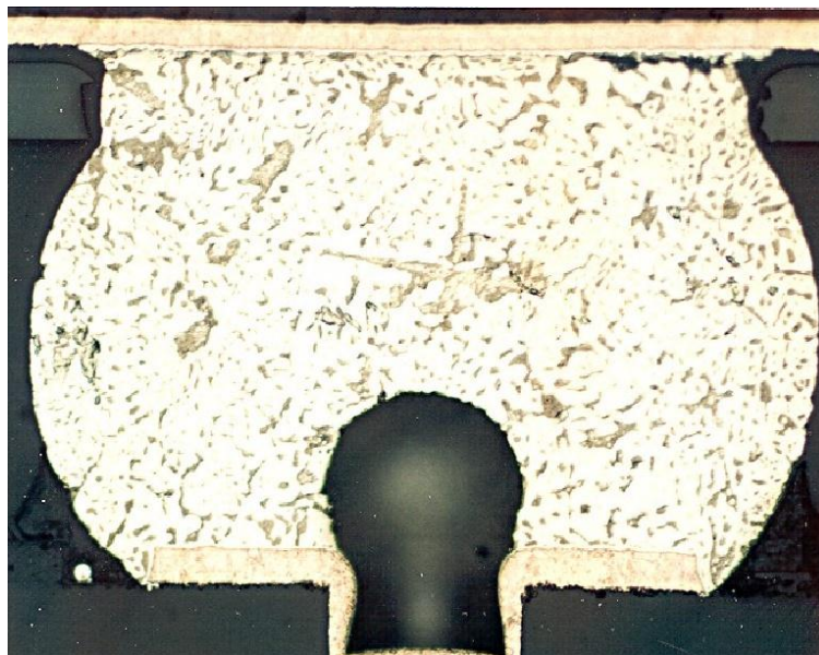
Figure 2: Example of a conformal microvia in pad and associated void in a SnPb assembly after thermal cycling. Fatigue crack is away from the void.
