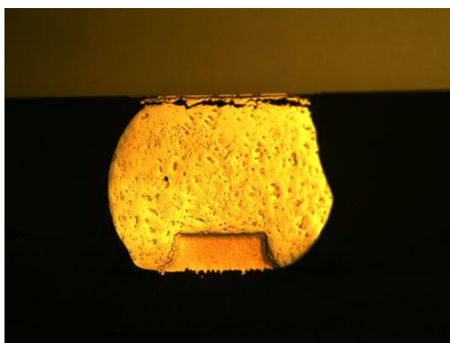
Figure 25: WSBGA 36, Assembled with SAC solder, failed at 1886 cycles in 0-100°C thermal cycling
