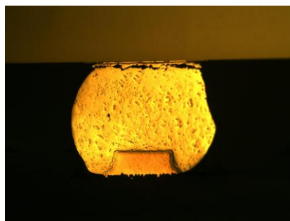
WSBGA 36, Assembled with SAC solder, failed at 1886 cycles in 0-100° C thermal cycling
