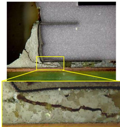
5 × 7 Ceramic Oscillator, assembled with SAC solder, failed at 1586cycles in 0- 100° C thermal cycling
