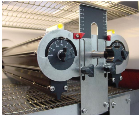
Figure 3 – Adjustable Air Knife Blower in Drying Section
