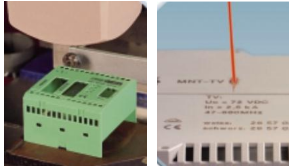
Figure 17: Pad and Laser Printing
