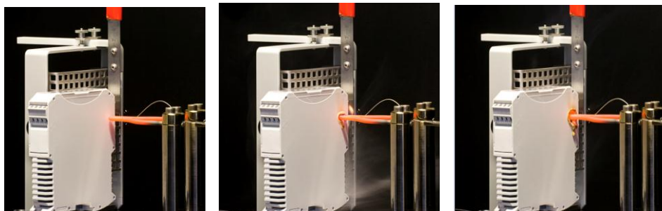
Figure 21: Glow Wire Test on Electronic Housing
