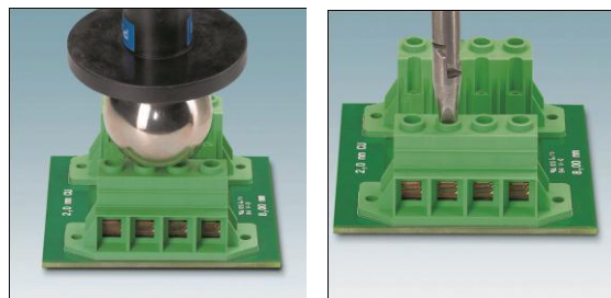
Figure 20: “Back of Hand” and “Finger” Safety Tests per IEC 60529
