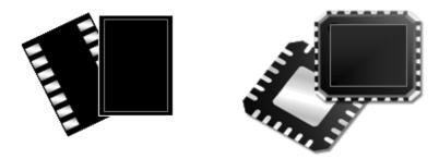
Figure 1. Comparing SON and QFN bottom termination semiconductor packaging.
