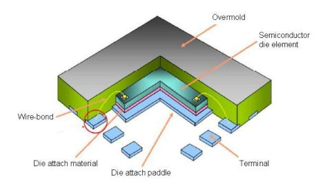
Example source: Texas Instruments Figure 5. QFN showing terminal contacts and DAP feature
