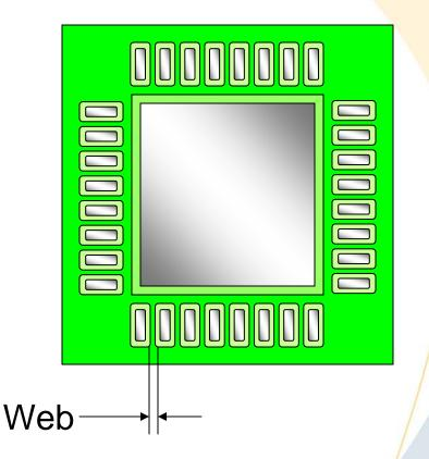
In general, the solder mask opening will be 120 to 150 microns larger than the PCB land pattern resulting in 60 to 75 micron clearance between the land pattern and soldermask.
