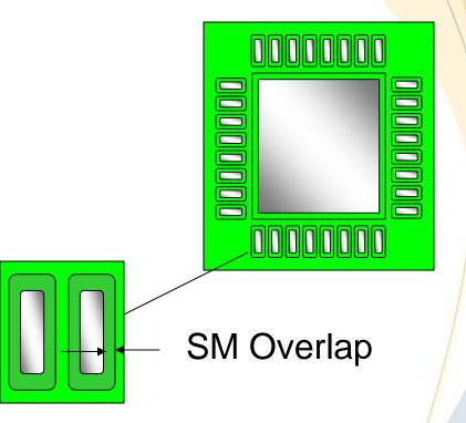
For SMD applications, the mask opening should be approximately 100 microns smaller than the land and thermal pad to overlap the land and thermal pad on all four sides.
