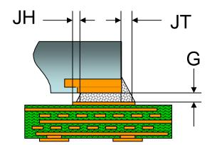
Solder fillet on coated or plated terminal end
