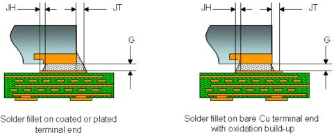
Figure 6. Comparing the solder fillet profile on QFN and SON terminal ends.
