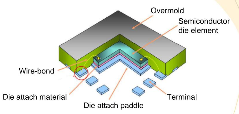
The exposed DAP serves to assist in transferring any thermal rise generated by the die element directly onto the host circuit structure.
