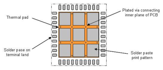
Figure 9. Segmented solder paste pattern with plated vias on thermal pad.
