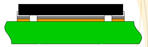
Rather than coagulating in the center of the thermal pad during reflow soldering, the partitioned solder pattern will maintain a uniform interface between surfaces.
