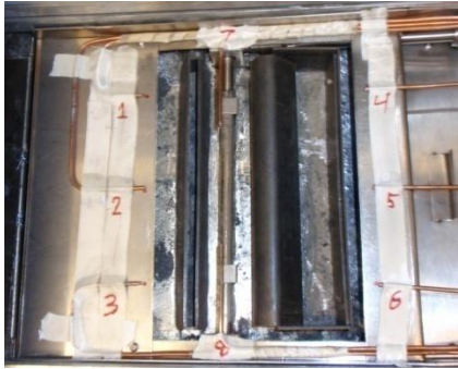
Figure 10 - Eight Sampling Tubes Around Solder Pot
