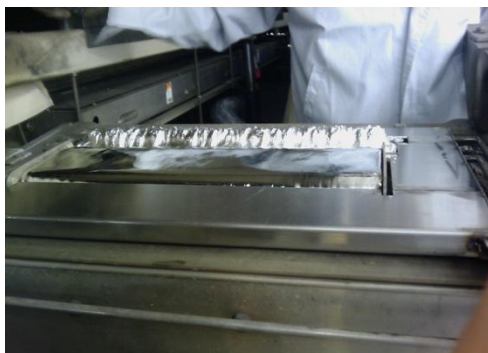
Figure 18 - Protective Housing Inserted in a Solder Pot with Two Waves
