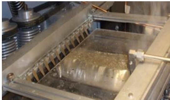
Figure 15 - Flux Vapor Generated from a Hot Flux Reservoir
