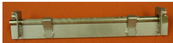
Figure 12 - A Metal Fin Mounted on the Middle Diffuser
