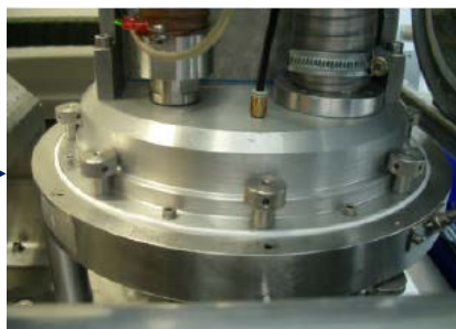
Vacuum Head Lowered into Solder Spheres Reservoir
