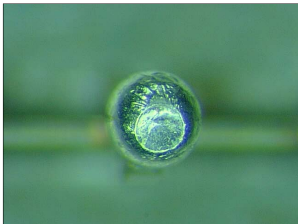
Head-in-Pillow Solder Joint (Solder Ball Side) – Solder Paste A
