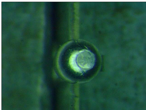
Head-in-Pillow Solder Joint (Solder Ball Side) – Solder Paste B
