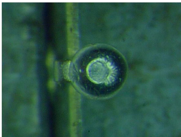
Head-in-Pillow Solder Joint (Solder Ball Side) – Solder Paste C
