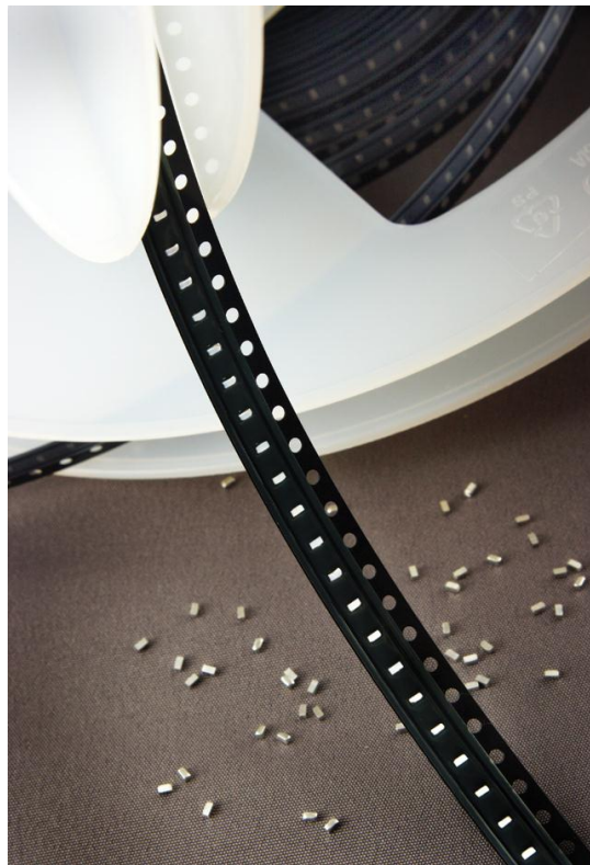
Figure 5. PIP preforms come in tape & reel feeder packaging.
