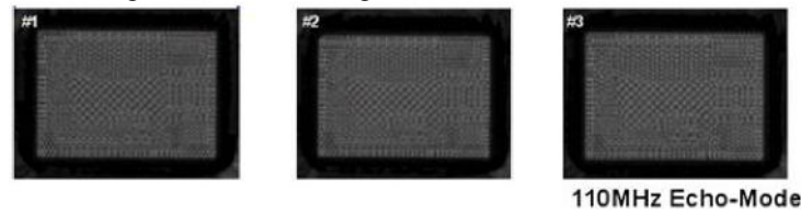
Fig. 22. Underfill void inspected by SAT.
