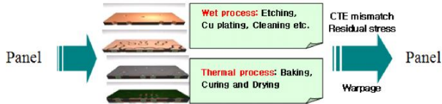
Fig. 5. Warpage derived from periodic work by heating and wet process in PCB fabrication.
